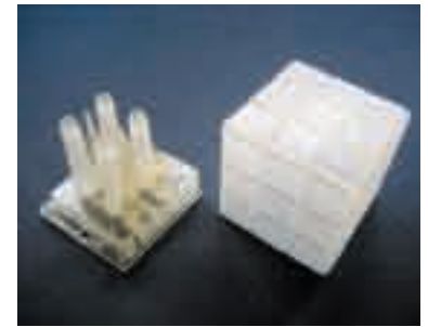
Figure 1: Prototype of an illuminated cube created on the Eden260™
